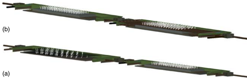
Figure 5.4 Presentations of Hybrid Systems: (a) FWSCWs-HSFCWs, (b) HSFCWs-VSFCWs.
