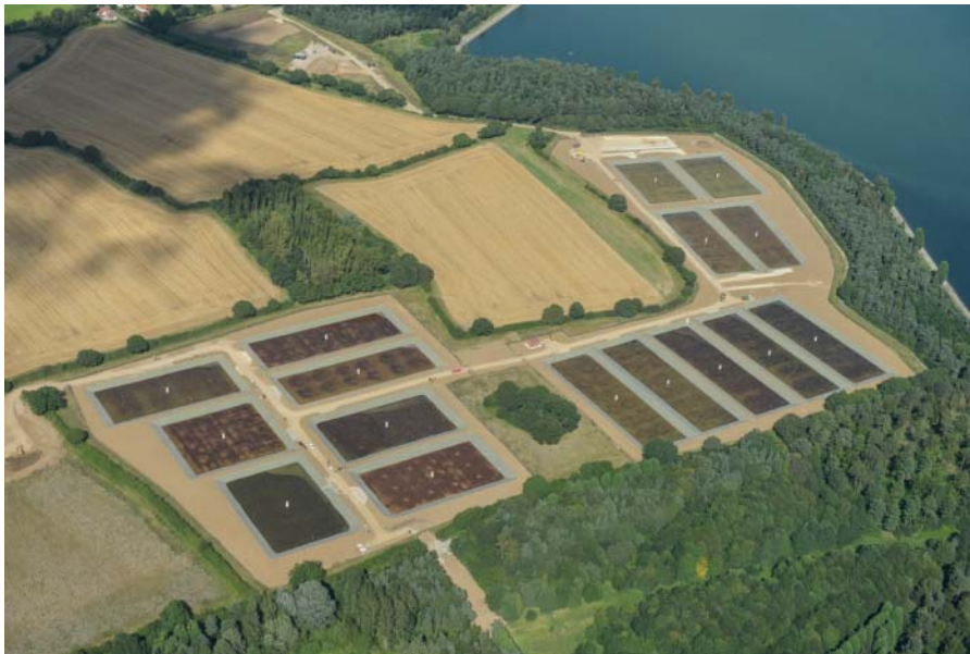
Figure 19.7 Hanningfield STRB system treating sludge from Hanningfield Water Works situated 3 km from the STRB (Photo: Orbicon September, 2012).
