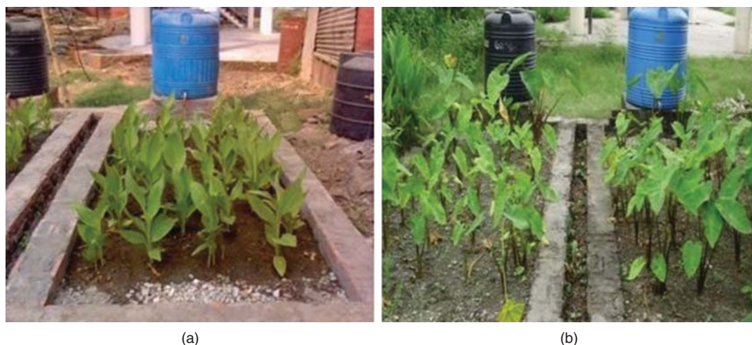
Figure 15.1 View of the experimental HSSF-CW. (a) CW planted with Canna indica , (b) CW planted with Colocasia esculenta .
